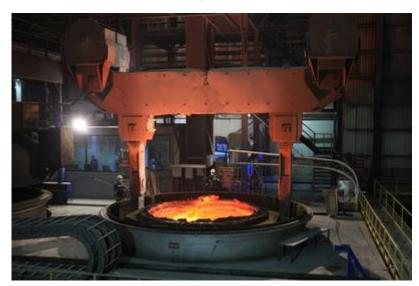
In the Dilovası meltshop of Turkish steelmaker Çolakoğlu Metalurji A.S. (Çolakoğlu), Primetals Technologies upgraded an existing VD(Vacuum Degassing) plant to a VOD (Vacuum Oxygen Decarburization) plant.
